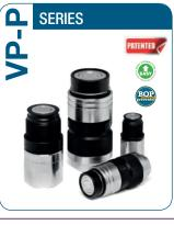
ving style: Flat face nterchange: Stucchi profile Available sizes: From 1/4" to 1-1/2" Operating pressure: Up to 600 bar Flow rate: Up to 750 L/Min Material: High strength carbon steel Connection system: Screw Connection under pressure: Both side, easy connection + disconnection allowed Typical use: **Outdoor**
