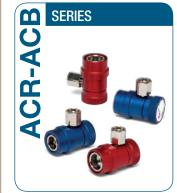
Valving style: Poppet Interchange: SAE J639 Available sizes: 1/4" Operating pressure: Up to 41 bar Material: Brass/Aluminum Connection system: Push - screw onnection under pressure: Not allowed vpical use: **Indoor**
