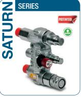
living style: Flat face Interchange: ISO 16028 (for the couplings) Available sizes: From 1/2" to 3/4" Operating pressure: Up to 350 bar Flow rate: Up to 200 L/Min Material: High strength carbon steel Connection system: Push onnection under pressure: One side + disconnection allowed (using Knob) Typical use: **Outdoor**
