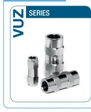
Valving style: Check valves Available sizes: From 1/8" to 2" Standard cracking pressure: Up to 4.5 bar Flow rate: Up to 1000 L/Min Material: High strength carbon steel Typical use: **Outdoor**
