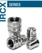
Valving style: Poppet Interchange: With similar product (Nordic interface) Available sizes: From 1/4" to 1" Operating pressure: Up to 300 bar Flow rate: Up to 378 L/Min Material: Stainless steel (AISI 316L) Connection system: Single acting sleeve Connection under pressure:
