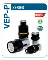
ving style: Flat face terchange: Stucchi profile Available sizes: From 1/4" to 2" Operating pressure: Up to 600 bar Flow rate: Up to 1000 L/Min Material: High strength carbon steel Connection system: Screw Connection under pressure: Both side, easy connection + disconnection allowed Typical use: **Outdoor**
