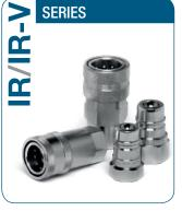
Alving style: **Ball/Poppet** Interchange: Similar couplings + IR V + ISO 7241-1 "A" size 1/2" only Available sizes: From 1/4" to 1" Operating pressure: Up to 300 bar
