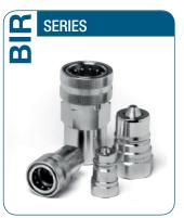
Valving style: Poppet Interchange: ISO 7241-1 A Available sizes: From 1/4" to 2" Operating pressure: Up to 350 bar Flow rate: Up to 1000 L/Min Material: High strength carbon steel Connection system: Single acting sleeve Connection under pressure: One side with PC version Typical use: Outdoor
