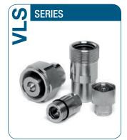
Valving style: Poppet Interchange: Similar Couplings Available sizes: From 1/2" to 1" Operating pressure: Up to 465 bar Flow rate: Up to 200 L/Min Material: High strength carbon steel Connection system: Screw Connection under pressure: **One side** Typical use: Outdoor
