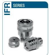
Valving style: Flat face Interchange: ISO 5676 Available sizes: 3/8" Operating pressure: Up to 150 bar Flow rate: Up to 23 L/Min Material: High strength carbon steel Connection system: Single acting sleeve Connection under pressure: Not allowed Typical use: Outdoor
