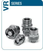
Valving style: Flat face limited spill Interchange: Similar Couplings (Rohrleitung) Available sizes: From 3/8" to 1-1/4" Operating pressure: Up to 420 bar Flow rate: Up to 576 L/Min Material: High strength carbon steel Connection system: Screw Connection under pressure:
